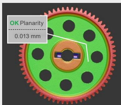
Flatness measurement of the flange of a gear wheel
