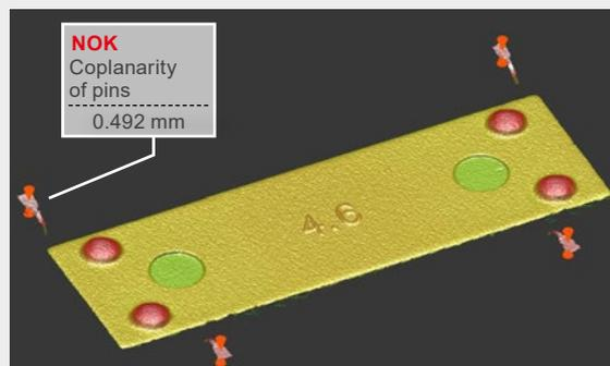
Coplanarity measurement of contacts on electrical components
