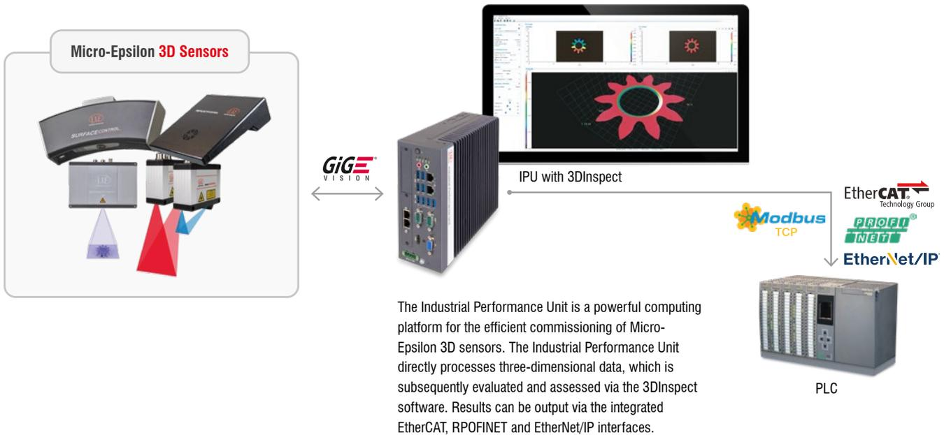
3DInspect is a uniform and user-friendly software tool for all 3D sensors from Micro-Epsilon. Parameter setting of the 3D sensors and recording of the measurement data are done directly in the 3DInspect software. Powerful tools allow point cloud alignment and filtering, intuitive detection and selection of relevant areas, and program combination. The 3D point clouds can be processed as required and measured values can be output to the controller.
