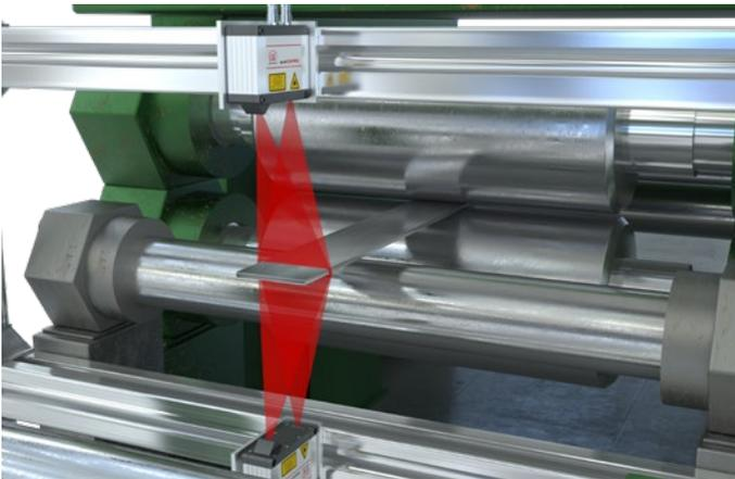
Thickness measurement of cold rolled steel strips
