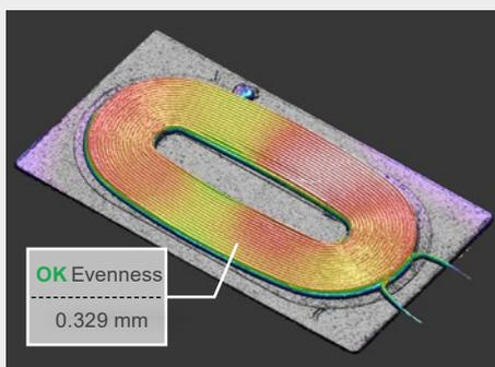
Flatness test of the winding on charging coils
