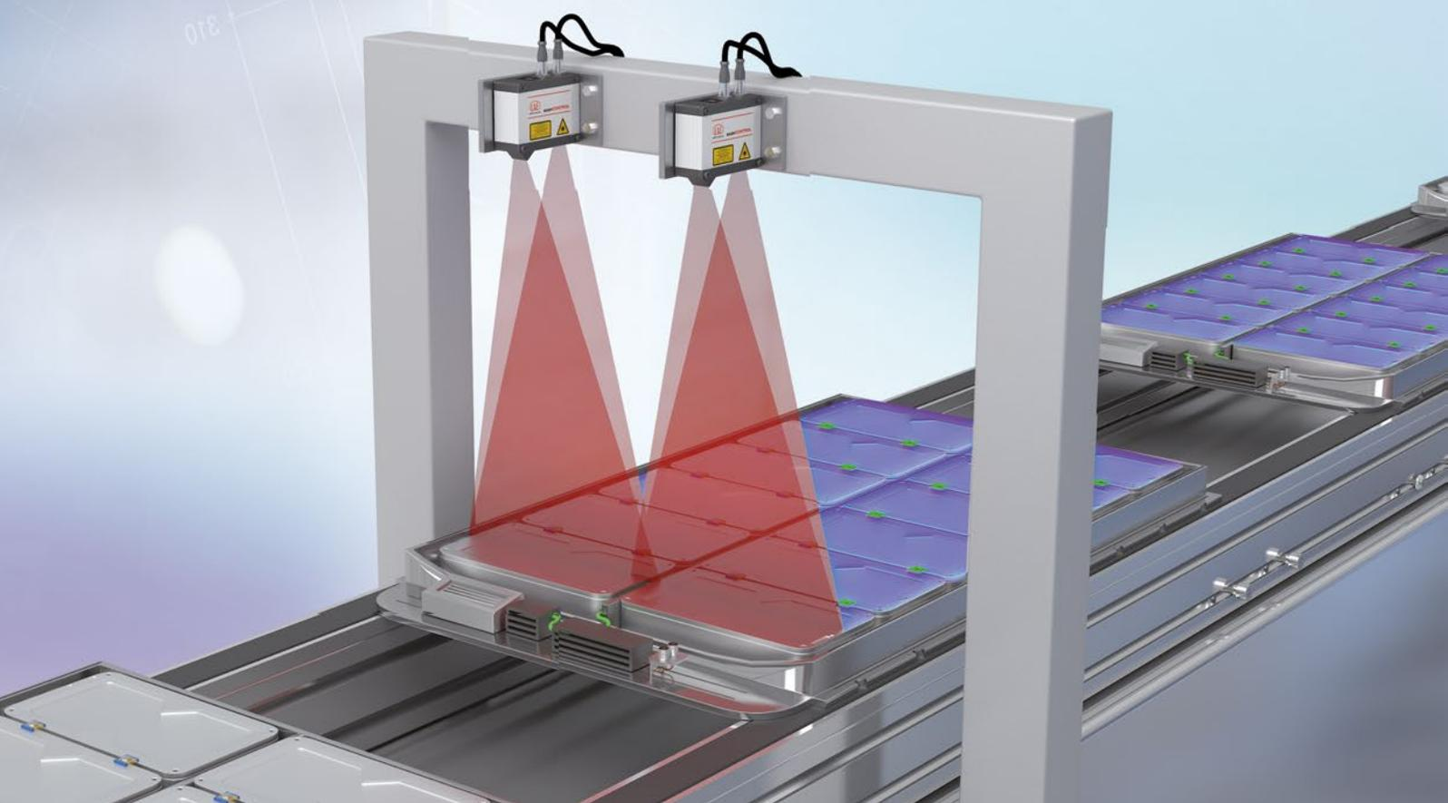
The 3D Profile Unit enables the calculation of several individual profiles of scanCONTROL 30xx sensors in a common coordinate system. This is how a composite 2D profile or a composite 3D point cloud can be generated. It enables the detection of various geometries, the extension of measuring ranges and the performance of thickness measurements.
