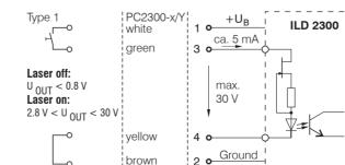
If pin Pin 3 with +U<sub>n</sub> and Pin 4 are not connected with ground, the laser is off.
