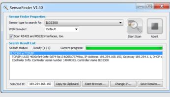
Alternatively: If DHCP is enabled and the DHCP server is linked with the DNS server, an access is possible on "ILD2300 SN01234567"
