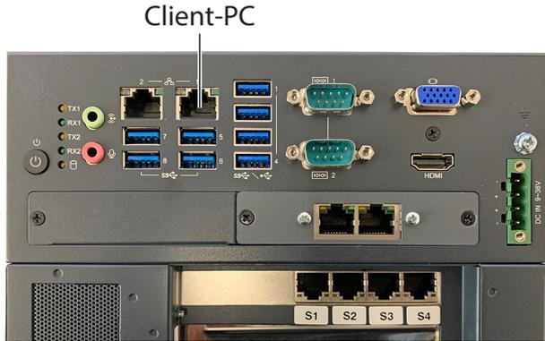
Fig. 19 Connecting client PC to Profile Unit Controller
