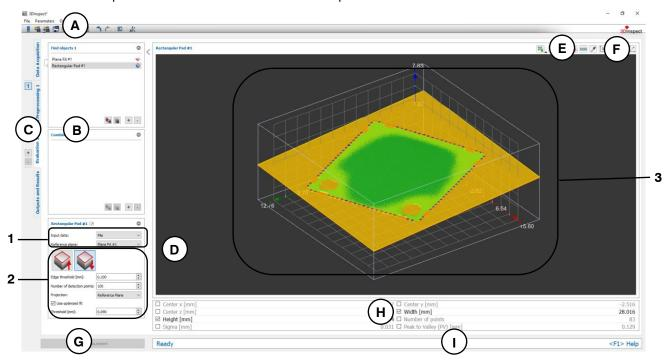
Fig. 6.12: "Rectangular Pad" Measuring Program
