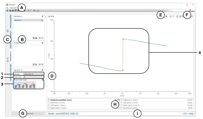
Fig. 6.28: "Gap 2D" Measuring Program
