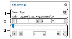
Fig. 3.18: Settings in offline mode – single file ("2D" data format)
