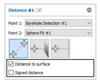
Fig. 3.75: Parameters for the "Distance" measuring program
