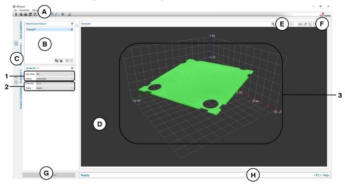
Fig. 5.17: "Closing" Measuring Program
