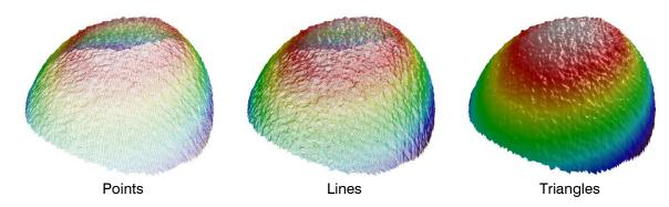
Fig. 3.40: Display methods for the 3D-View
