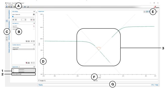
Fig. 6.38: "Angle 2D" Measuring Program
