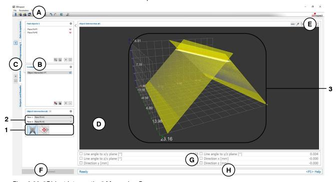
Fig. 6.32: "Object Intersection" Measuring Program
