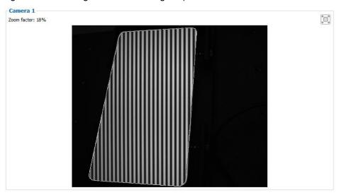
Fig. 3.7: Positioning the reference target – position is OK
