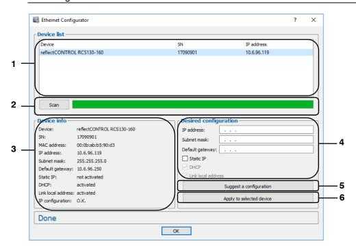
Fig. 3.90: "Ethernet Configurator" dialog box
