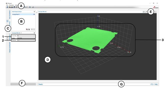
Fig. 5.13: "Average Filter" Measuring Program
