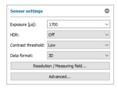
Fig. 3.11: "Sensor settings" box (surfaceCONTROL)
