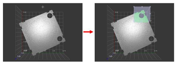
Fig. 3.63: Setting the complete ROI (x/y range)
