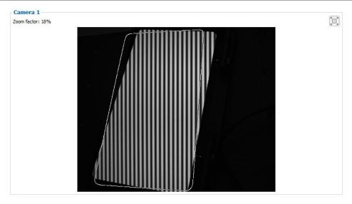
Fig. 3.6: Positioning the reference target - position has to be corrected
