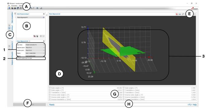
Fig. 5.6: "Plane Alignment" Measuring Program
