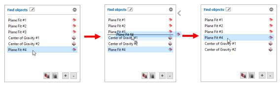
Fig. 3.53: Moving a measuring program
