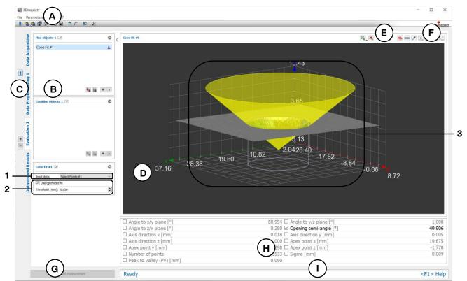
Fig. 6.8: "Cone Fit" Measuring Program
