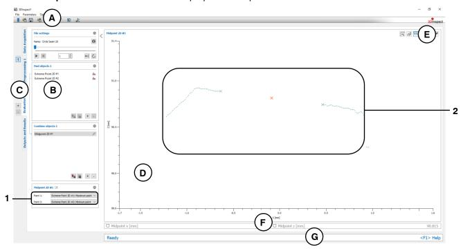
Fig. 6.40: "Midpoint 2D" Measuring Program
