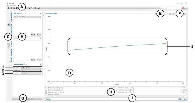
Fig. 6.18: "Extreme Point 2D" Measuring Program
