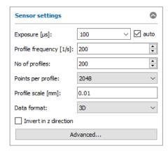
Fig. 3.12: "Sensor settings" box (scanCONTROL 30XX)
