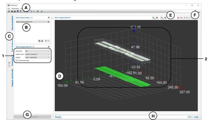
Fig. 5.21: "Wave Compensation" Measuring Program
