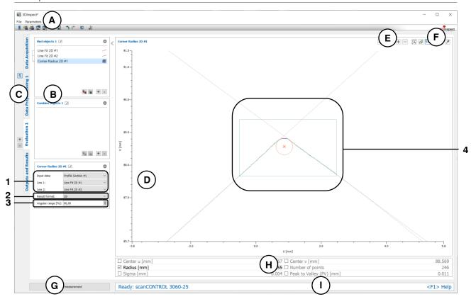
Fig. 6.21: "Corner Radius 2D" Measuring Program
