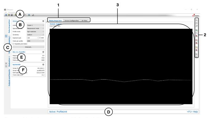
Fig. 4.3: "Display Image Data" view (3D Profile Unit)
