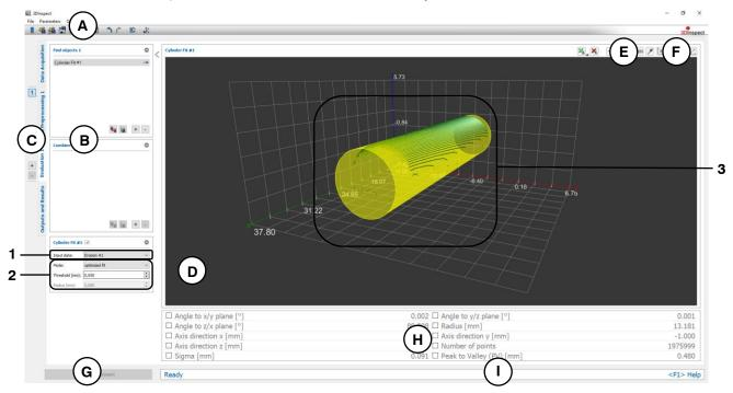
Fig. 6.7: "Cylinder Fit" Measuring Program
