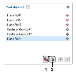
Fig. 3.54: Duplicate measuring program / Move measuring program to another program group
