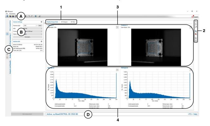
Fig. 4.1: "Display Image Data" view (surfaceCONTROL/reflectCONTROL)
