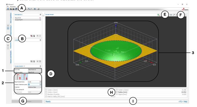
Fig. 6.10: "Circular Pad" Measuring Program
