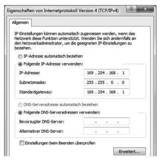
By default, the IP address of the controller is set to 169.254.168.150. Communication with the controller is done on the data port 10001 for measurement transmission. A command port (Telnet, port 23) is used for sensor commands.
