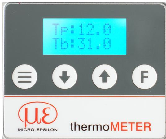
Fig. 7.1: Display and programming keys
