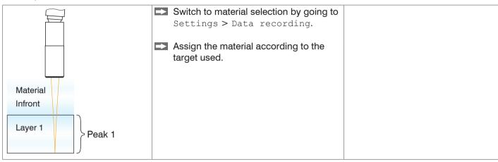
You can edit or add to the material table. For a new material, a group refractive index is required.
