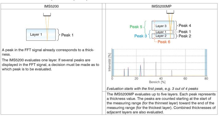
In the case of a target consisting of several transparent layers, the material must be assigned for each layer. The material selection for a thickness measurement starts with the thinnest layer (layer 1) independent of the physical arrangement in the measuring object, see Chap. Material Selection.
