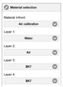
The IMS5200MP controller can also measure the thickness of combined layers of the same material.
