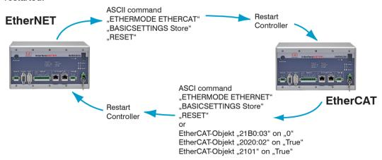
The RS422 interface for sending an ASCII command is available both in Ethernet mode and in EtherCAT mode.
