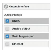
Selecting the required interfaces for data output
